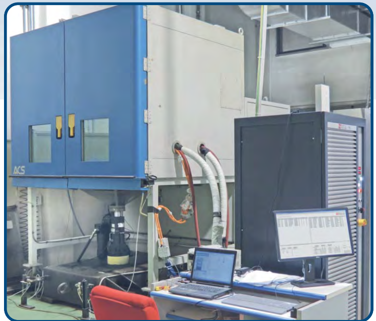
Test bench of the company Digatron for electric vehicle batteries
